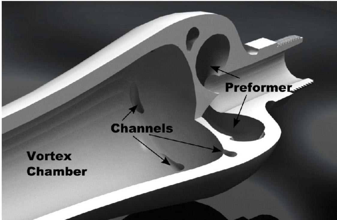
**Figure 1: The Watreco vortex generator with trumpet-shaped vortex chamber.**
